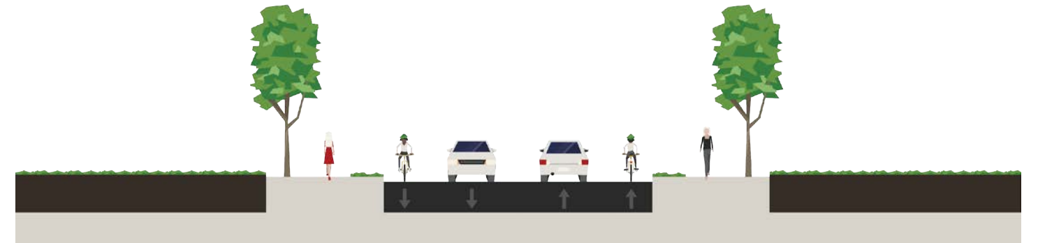
Illustrative rendering of 2 Lane Undivided with Curb and Gutter, Bike Lanes, and Sidewalks
