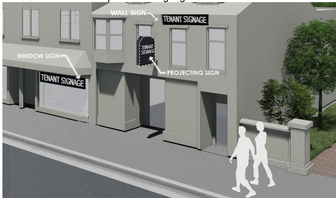
Figure B.3.3 Illustrative Example of Building Signs
