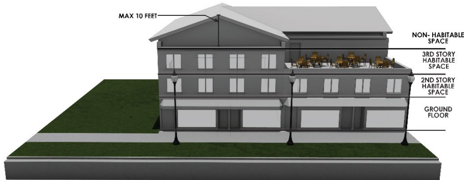
Figure B.2.3 Building Height Illustrations
